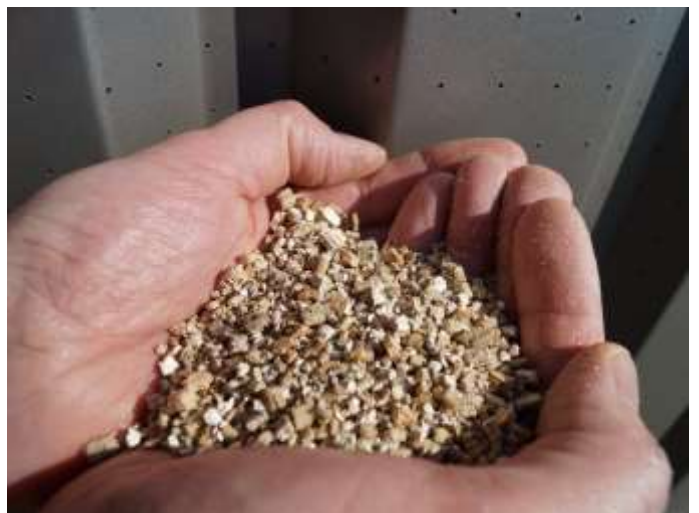
Figure 5.6: The thermochemical storage material
