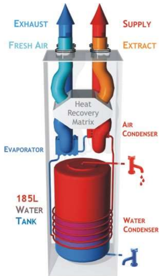
Figure 2.4: Cross section through a Genvex Combi 185 unit
