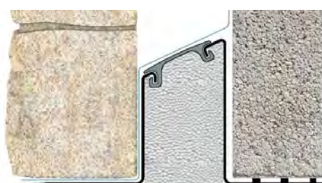
Figure 9.1: Illustration to show how Schöck Isokorb® minimises thermal bridging (Credit: Schöck)
